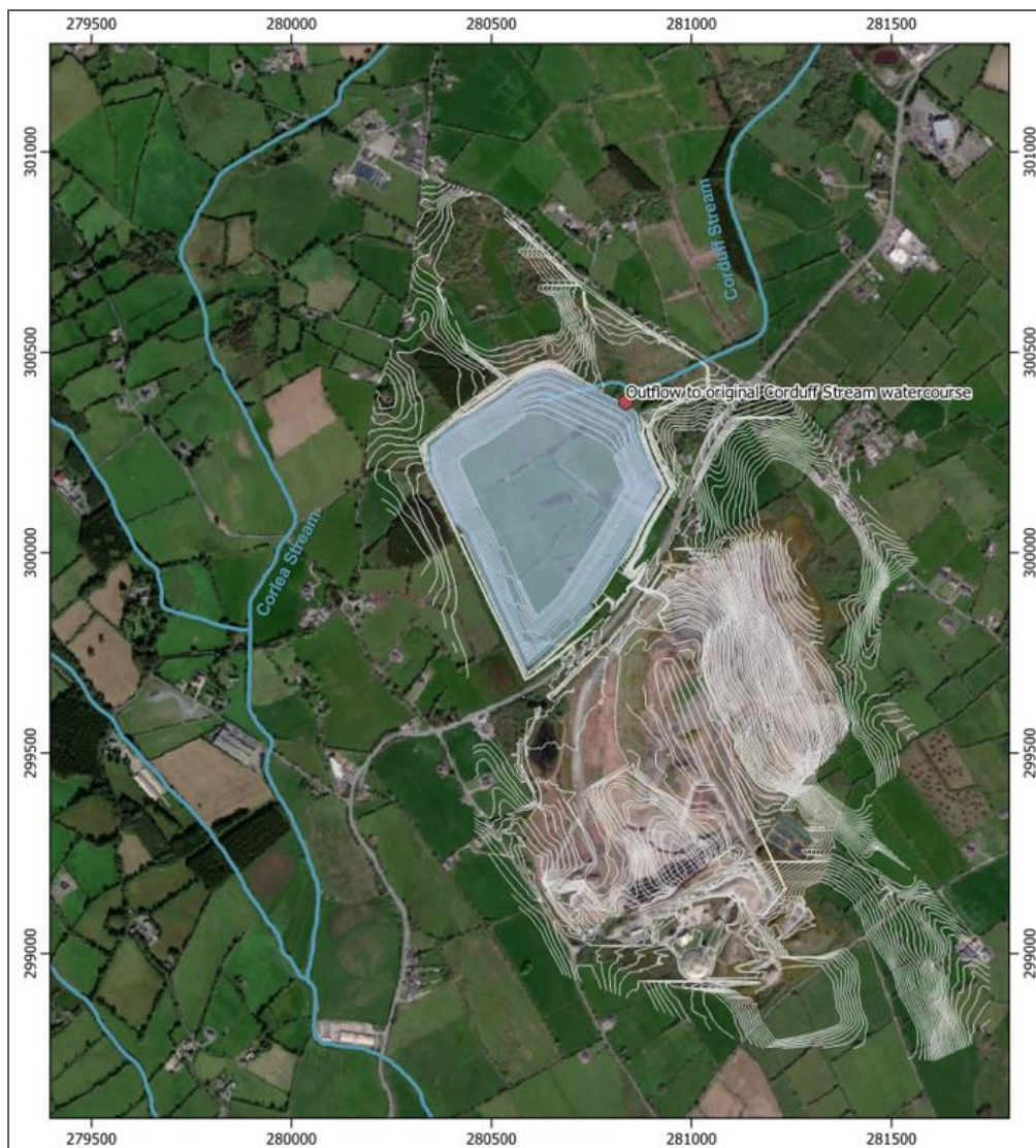
Figure 11 Final Knocknacran West water body with discharge from the eastern pit rim to the original Corduff Stream
