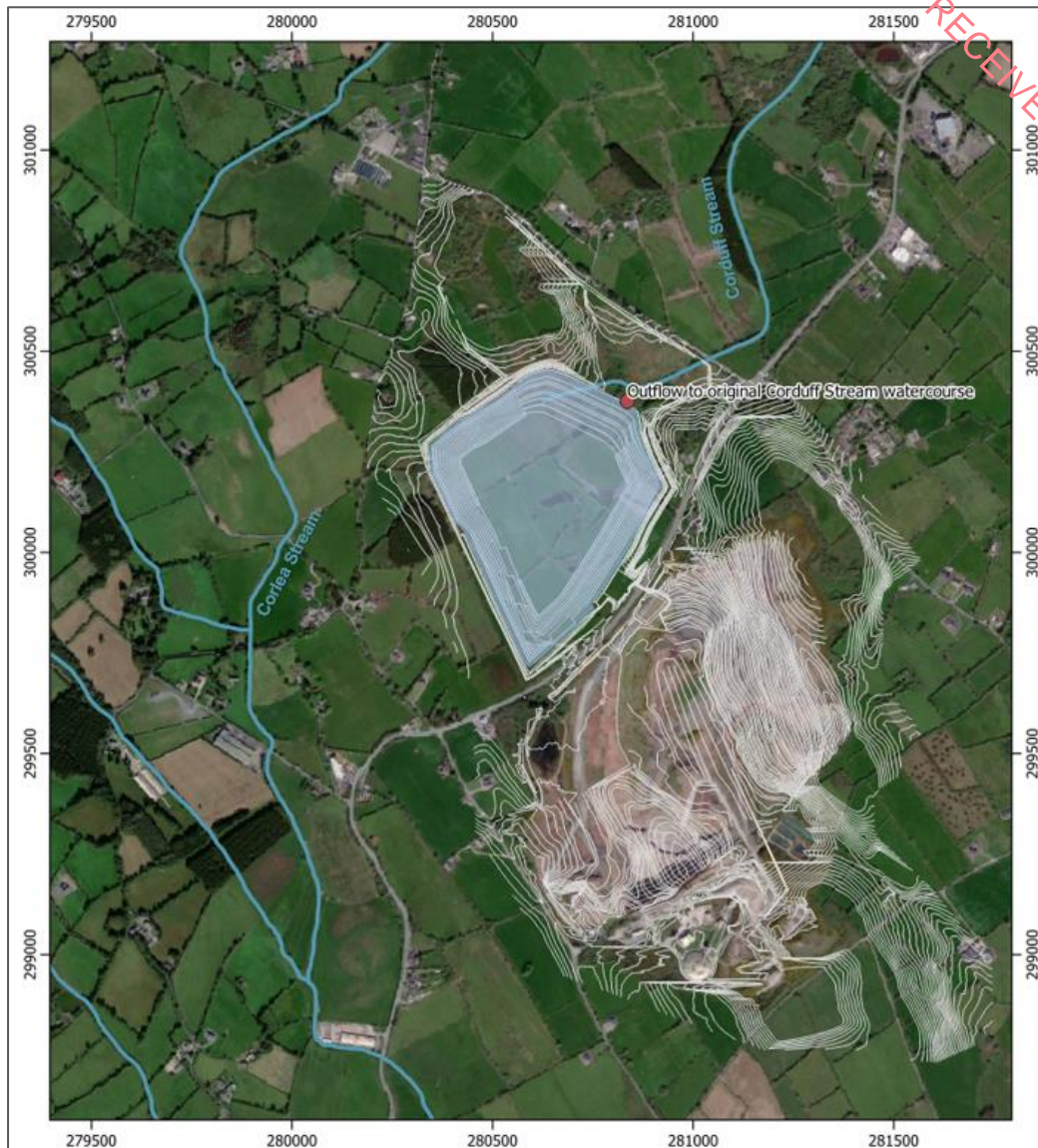
Figure 5: Final Knocknacran West pit lake with discharge from the eastern pit rim to the original Corduff Stream
